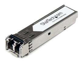
The 455886-B21-ST is a HP 455886-B21 compatible fiber transceiver module that has been designed, programmed and tested to work with HP brand switches and routers. It delivers dependable 10 GbE connectivity over fiber cable, for 10GBase-LR compliant networks, with a maximum distance of up to 10 km (6.2 mi).
